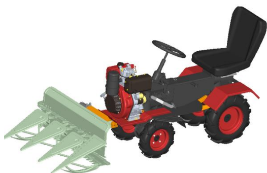
Fig. 1 – Overall highland barley harvesting and binding machine
